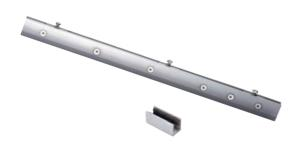
Applicable glass thickness: 10~12mm Standard product shipping length: 1,000mm Bearing≤160Kg
