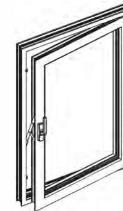
★ Positioning Micro ventilation state
