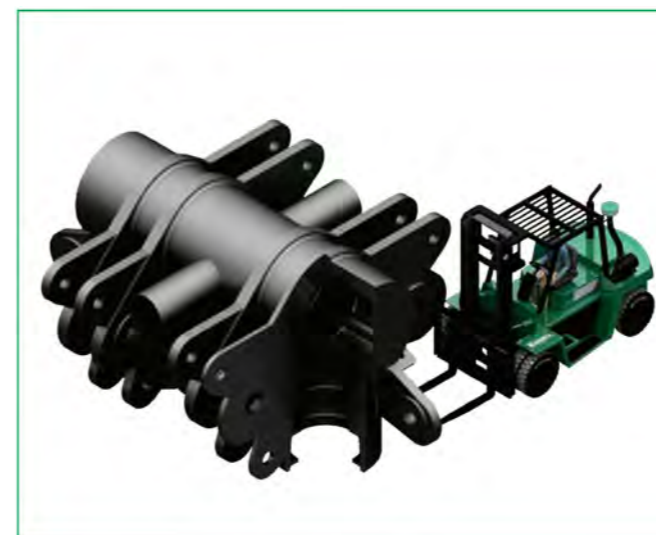
Big multi-cable confluence joint (weight:48t/pcs)
