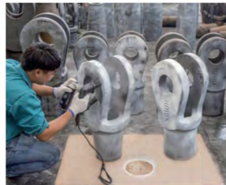
Magnetic particle inspection
