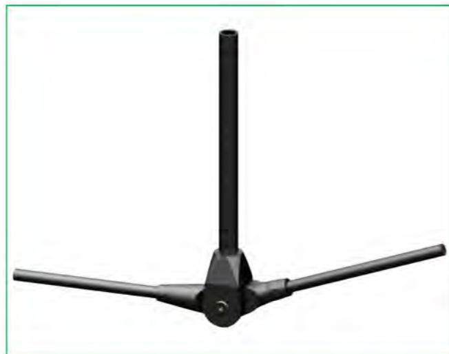
Lower chord structure support joint
