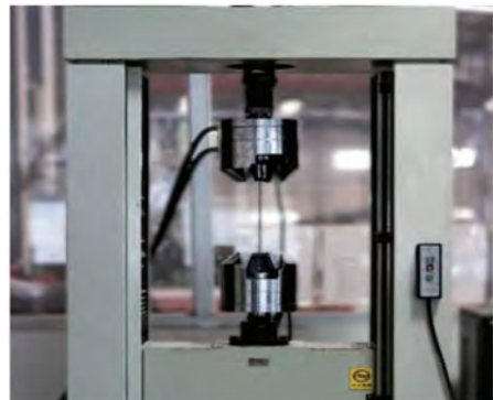
Tensile Testing for Steel Wire
