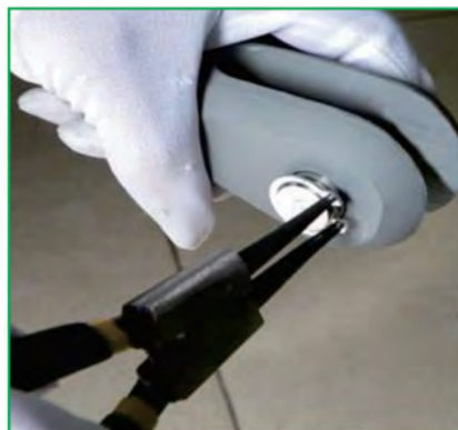
U-shape circlip installation drawing
