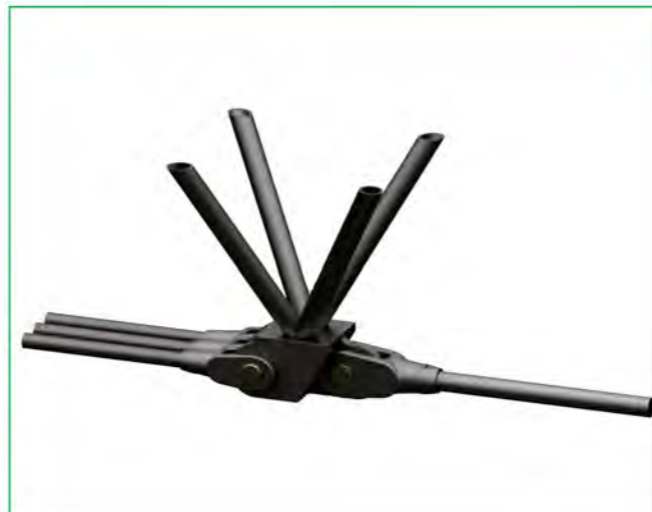
Lower chord structure support node
