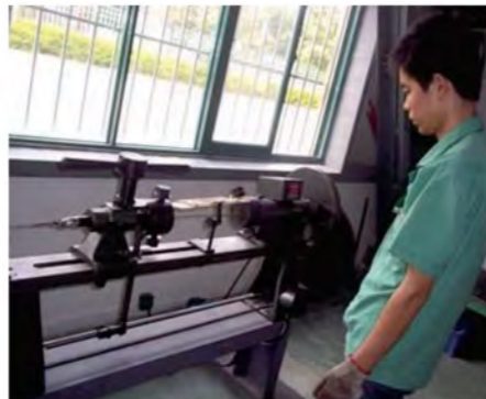
Torsion Testing for Steel Wire
